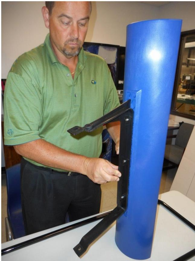
Insert three (3) - 1" X 5/16" carriage bolts through face of blade into holes in the mating bracket. Be sure to align the square portion of the bolt head with the square opening in the face of the blade.
