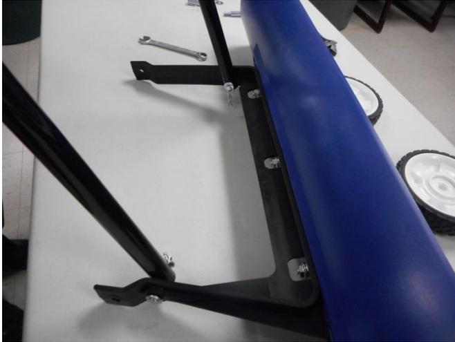
Secure clevis pin with one (1) - 1/4" flat washer followed by the key ring. Repeat the clevis pin insertion on the other side of the bracket and secure using the key ring using the same components.
