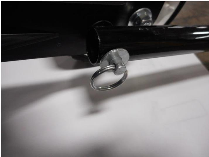
Make sure that the split ring is fully inserted into the clevis pin.
