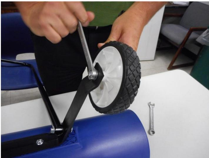
Tighten nuts using the 9/16" wrench and the adjustable wrench to hold both the bolt head and nut during the tightening process. The self-locking nut will require more force to tighten than a standard nut.
