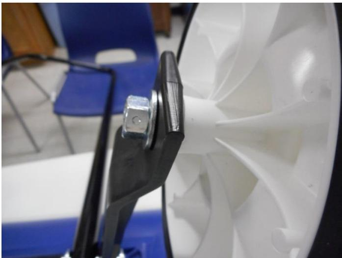
This is a properly tightened locking nut. Excessive wheel vibration can occur if the nuts are not properly tightened. Repeat same process for the other wheel.
